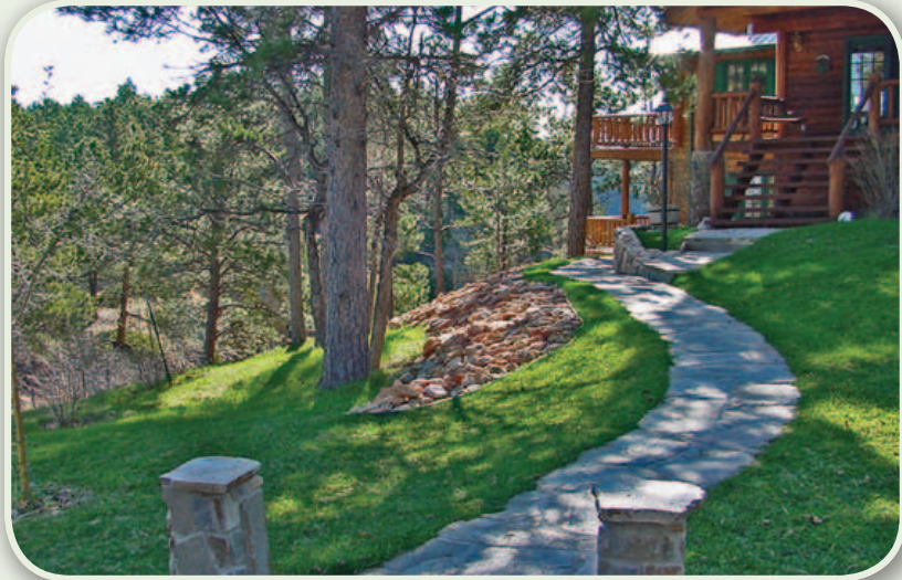
Fire burns faster uphill, making the removal of vegetation farther out essential to slow the fire down.
